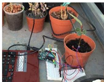
**Figure 6** Measuring soil humidity with two nails
