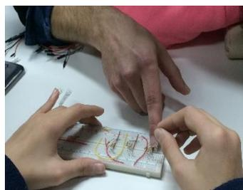
**Figure 5** Building the circuit board on the breadboard
