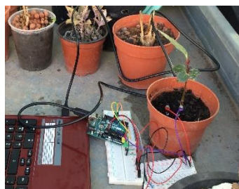
Figure 6 Measuring soil humidity with two nails
