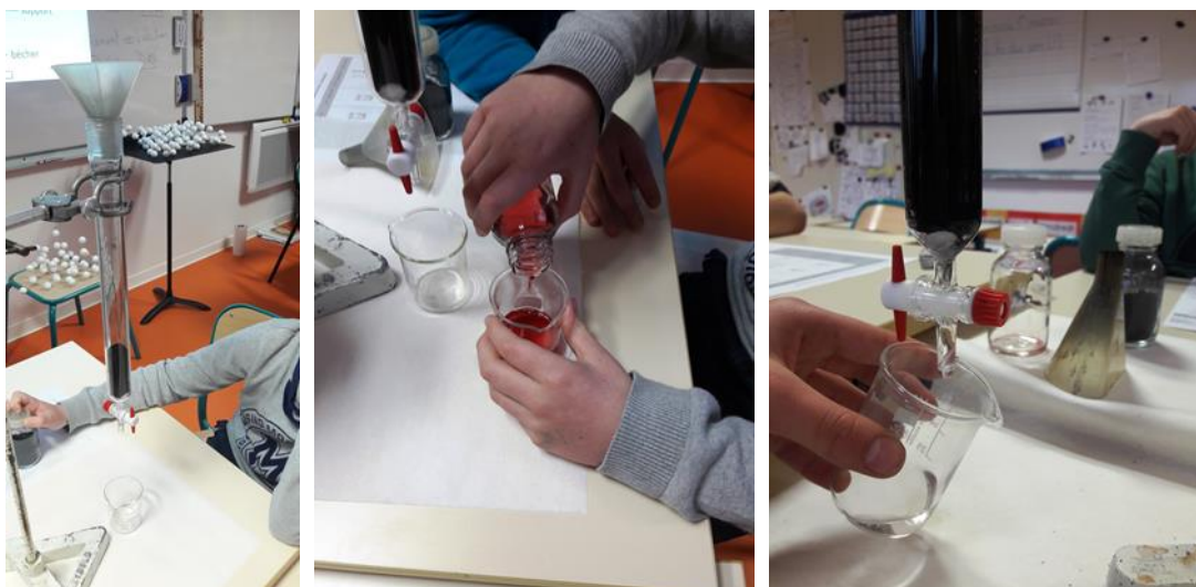
Figure 5 From left to right, steps of the experiment protocol: set up of the equipment, preparation of the column and grenadine solution, colorless filtrate.
